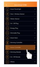
8. Proceed by pressing on "Search" to allow the ERIA hub to find the remote, the LED indicator on the hub will flash green this indicates that the hub is searching for new devices.
